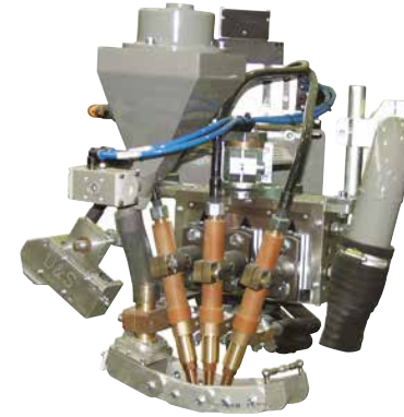
Helical or circumferential welding
